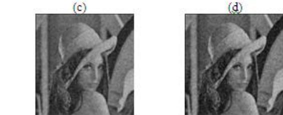
**Figure 5.9 (a) original image,(b) 2% Gaussian noise added to the original image.(c) Denoised image using standard mean filter.(d) Denoised image using Bit-plane method**
