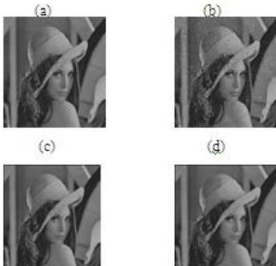
**Figure 5.1 a) original image (b) 2% salt and pepper noise (c) denoised image using Bit-plane method. (d) denoised image using Bit-plane method.**
