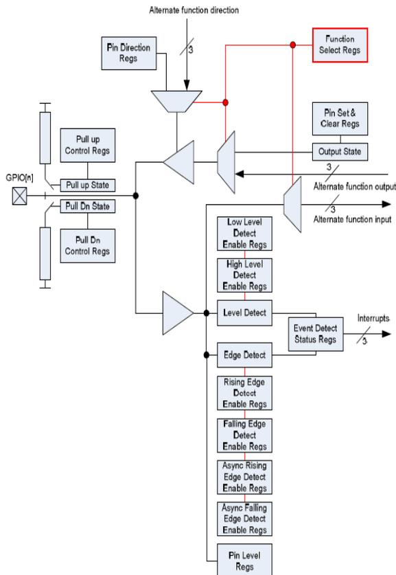
Fig 2.9: GPIO block diagram
