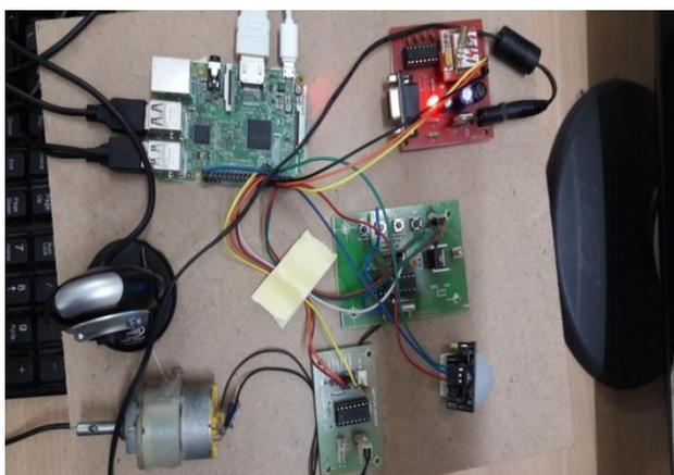
**Fig 5.2: Proposed transmitter**
