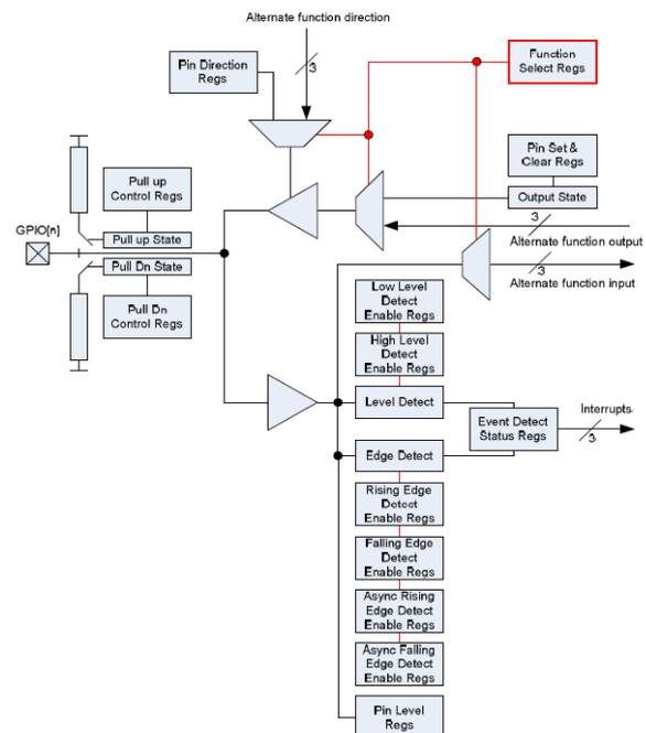
Fig 2.5: GPIO block diagram
