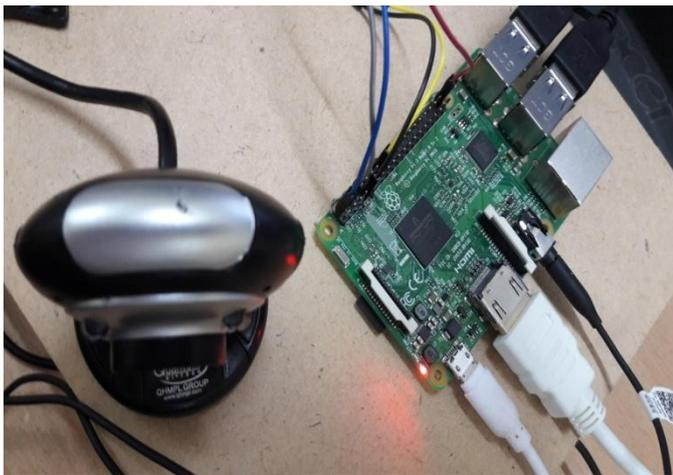
Fig 5.5: Interfacing web camera with Raspberry pi
